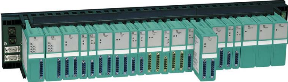
Fig. 2: Ethernet Remote I/O showing redundant gateways
